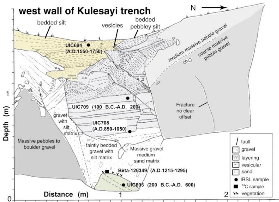
Figure 3. Trench log of Kulesayi site. See text for explanation. IRSL is infrared stimulated luminescence.
